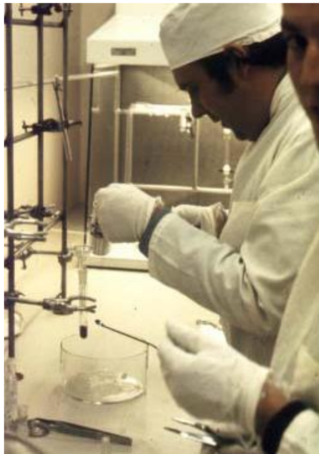
Above: James Maxwell transfers lunar dust (blackish material in test tube) from the special container used to ship it from Houston. All transfer operations were conducted in the Clean Air Facility in the basement of Chemistry, provided for the Apollo work. We managed to keep terrestrial organic contamination by, for example, skin lipids, plasticizers and lubricants to very low levels indeed.
